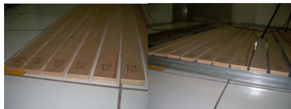
Figure 3. Spacings: 0mm, 3mm, 6mm, 9mm, 12mm, 15mm
