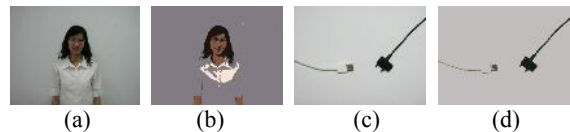
Figure 4. Background not contrast with the object: (a) Original 1, (b) Segmentation result of (a) (k=10, time=5647 ms), (c) Original 2, (d) Segmentation result of (c) (k=14, time=9172 ms)
