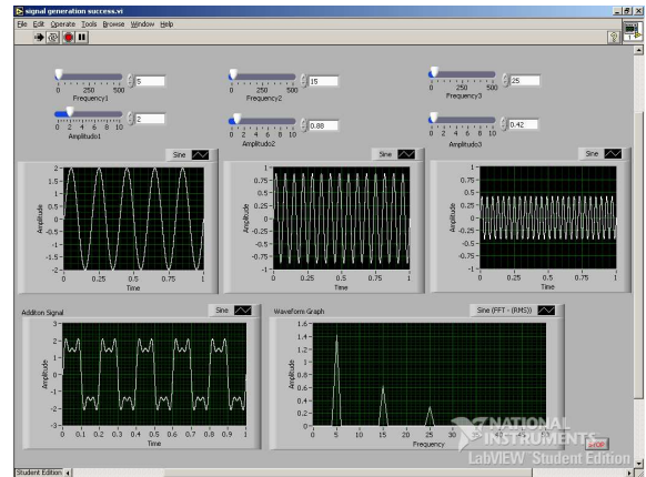
Figure 5 Signal making by combining the sinusoidal waves
