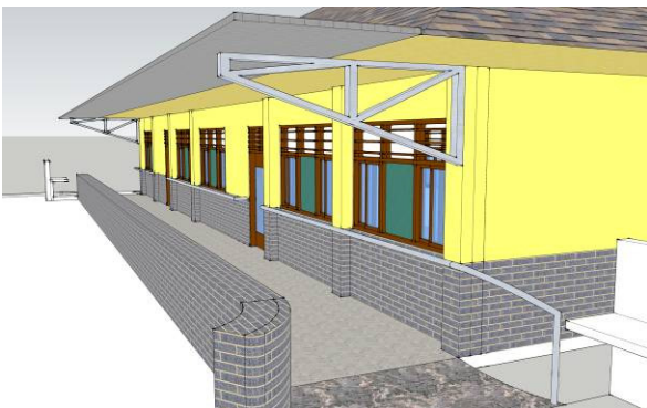
Figure 14. Proposed Additional Roof Canopy.
