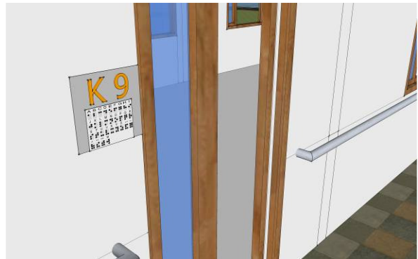
Figure 21. The classroom name signage with a regular letter and braille letter as high as 150 cm in the left of the door.
