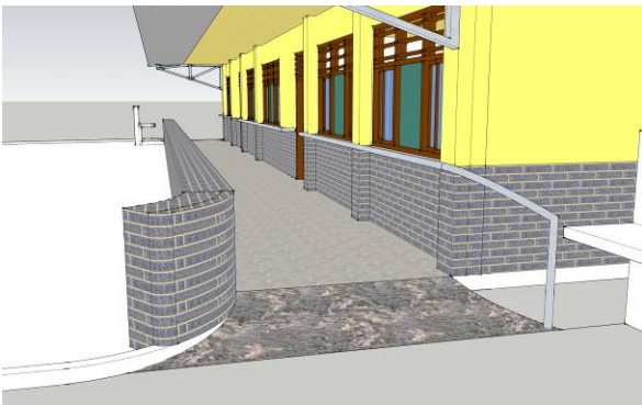
Figure 13. Proposed Ramp and Railing.
