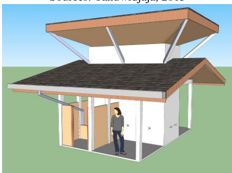
Figure 4. the Perspective of Integrated Bathing - Washing - Toilet - Water Tank Facility.
