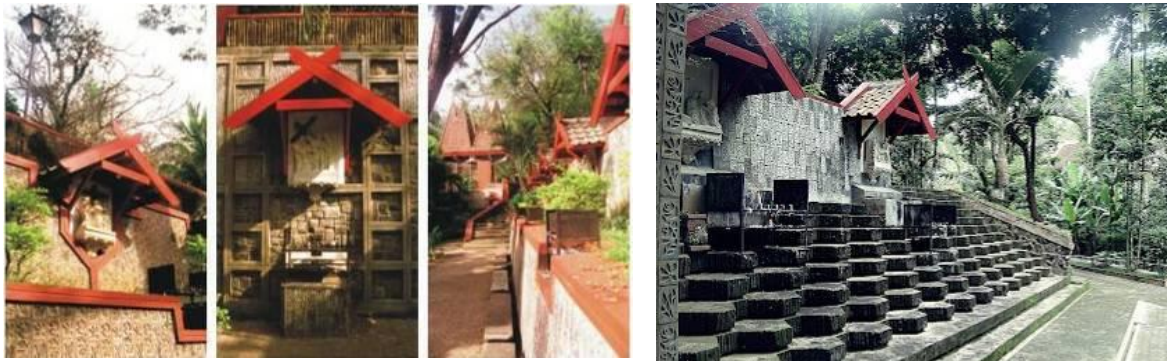
Figure 3. Contour of the ground, up and down, followed without making cut and fill, finished with simple materials
