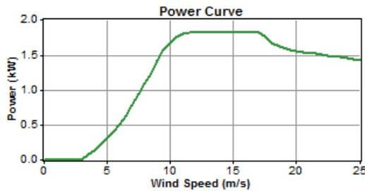
Fig 3: Power curve of a 1.8 kW wind turbine
