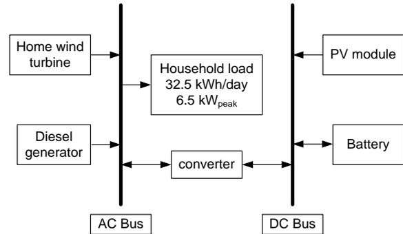
Fig 2: System configuration in complete option
