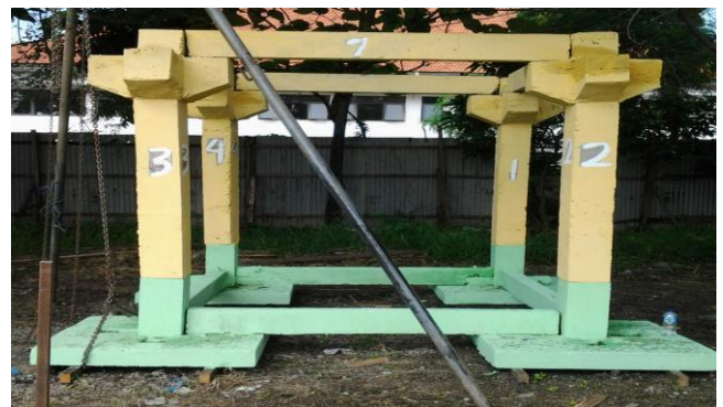
Figure 1. Prototype of column and beam connection
