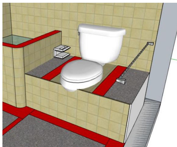
Figure 6. The Flexible toilet bowl for squatting and sitting for YPAB Blind School's Toilet Design
