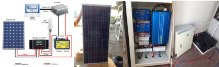
Fig. 10. Photovoltaic module with inverter and battery
