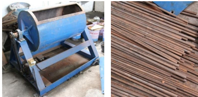
Figure 1: Rod Mill used for grinding the material
