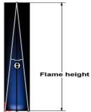
Figure 2: Measurement of Flame angle (θ) and flame height
