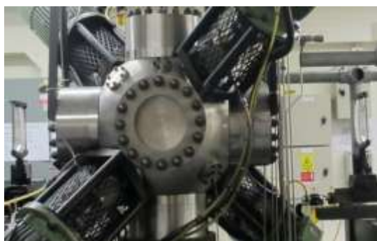
Fig. 3. 380mm diameter of Mk2 spherical bomb
