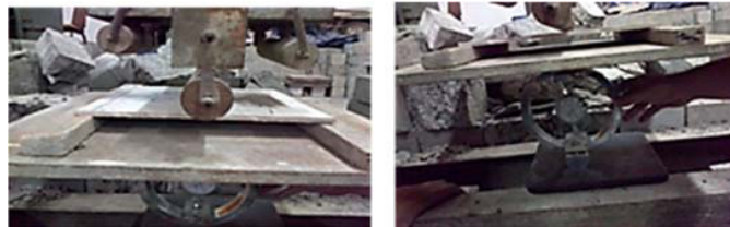
Fig. 2. Flexural strength test with proving ring machine
