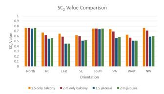
Figure 8. SC<sub>2</sub> (shading device only) Comparison Chart
