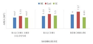
Figure 10. Average Depth of Penetration Area Comparison Chart
