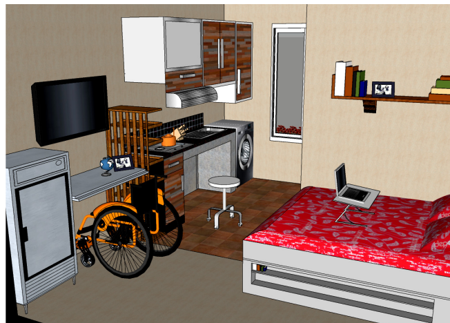
Fig. 7. Working area and pantry area that adjusted for wheelchair users. The spaces underneath the counter were provided for wheelchair users movement.
