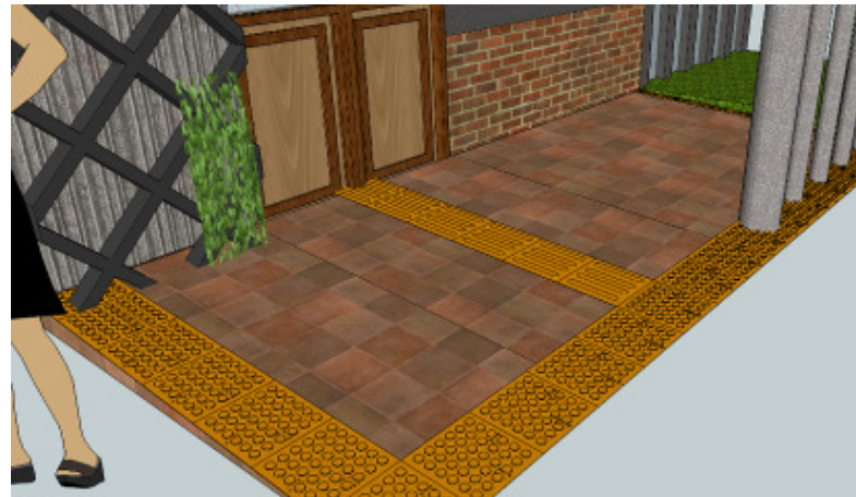
Gambar 75. Detail Guiding Path di Teras
