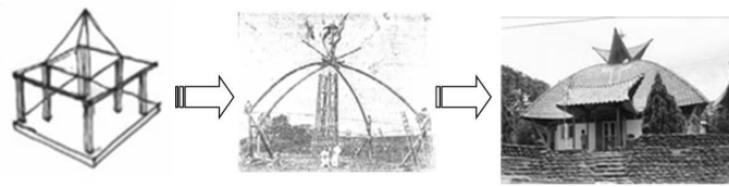
Figure 6. Photo of the transformation process from Javanese construction to Puhsarang church construction (Source: Maria I Hidayatun documentation, 2005).
