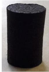
Figure 2. Briquette from Pterocarpus indicus leaves waste
