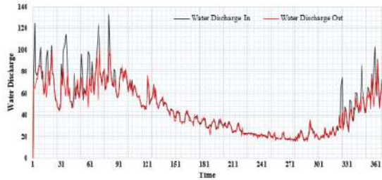
Figure 3: Comparison between Incoming Water Discharge and Outflow Water Discharge of Sengguruh Hydroelectric Power Plant
