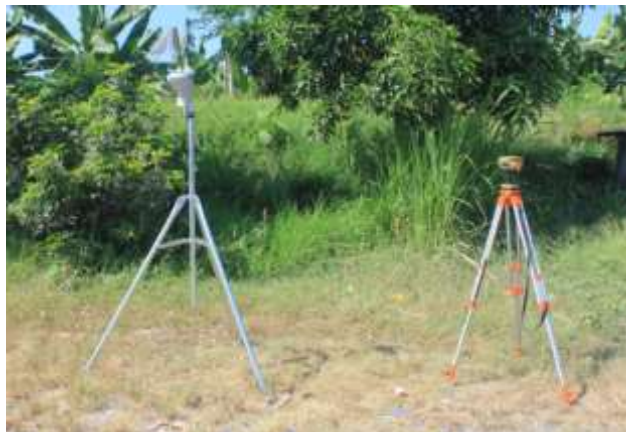
Figure 2. Installation of Geodetic Receiver and Weather Station in Tanjung Sari
