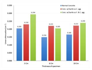
Fig. 5. Linear attenuation of concrete specimen fc'25
