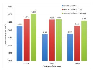
Fig. 6. Linear attenuation of concrete specimen fc'35
