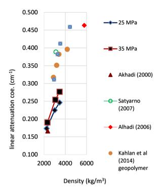
**Fig. 7.** Relationship between linear attenuation coefficient and density
