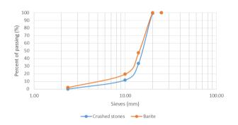
Fig. 1. The gradation of fine aggregates
