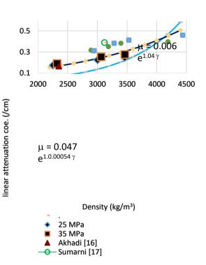
Fig. 8. Correlation between linear attenuation coefficient and material density, and proposed expression
