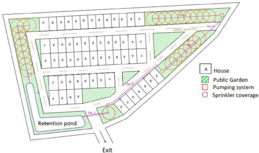
Figure 1: Lay out of the real estate with eco-drainage system (not to scale)
