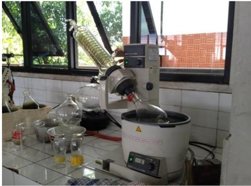
Gambar 2. Rotary evaporator.
