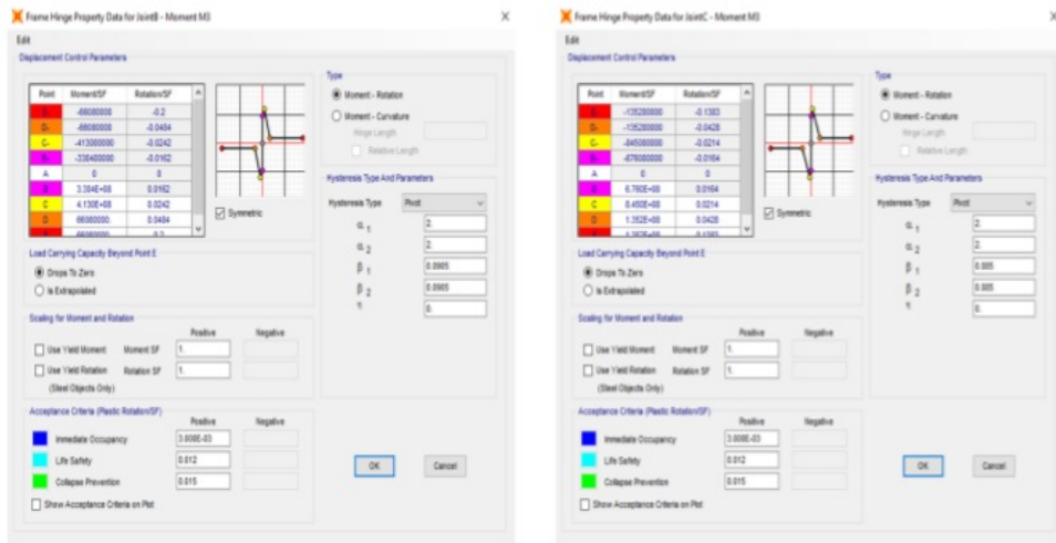
Figure 6. M3 hinges definition for joints (a) attached to beams (b) attached to columns
