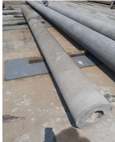
Figure 3. Precast Pile Specimens
