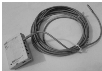
Figure 2: HOBO U Family Data Logger and External Water or Soil Sensor
