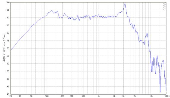
Gambar 9. Spektrum Analyzer Middle Speaker
