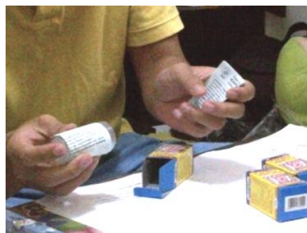
Figure 5. Operator holds leaflets in her left hand along the pillbox packaging process
