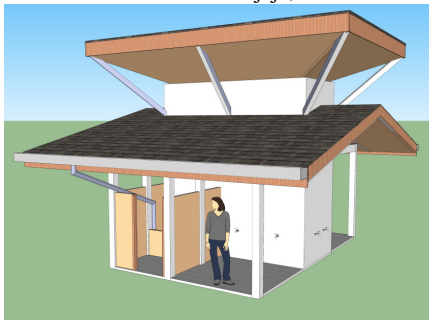
Figure 4. the Perspective of Integrated Bathing - Washing - Toilet - Water Tank Facility. Sources: Tanuwidjaja, 2013.
