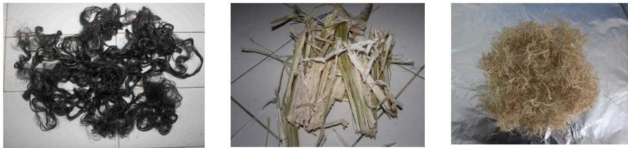
a) b) c) Figure 1 Materials used to make composite samples a) PP, b) as-received bagass fibres, and c) treated bagasse fibers
