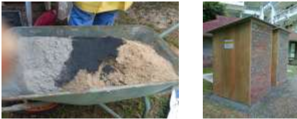
Figure 10. Designed test chamber to test on the coating material
