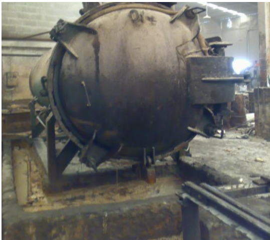
Figure 1. Autoclave using four key bolts
