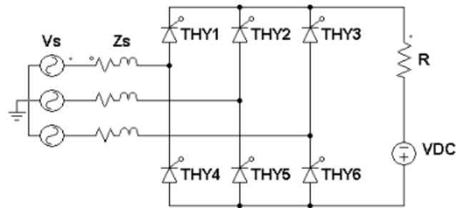
**Gambar 2.1. Line-commutated inverter**
