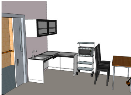
Fig. 14 The Kitchen Area, with clearance for wheelchair, anti-slip flooring and reachable sink and table top.
