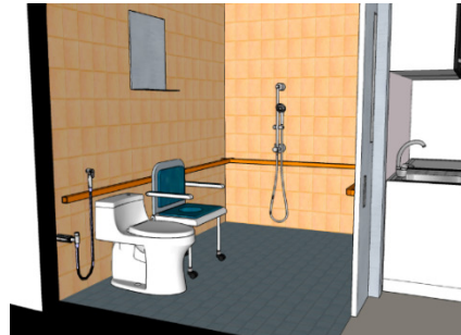
Fig. 15 The Bathroom, with sliding door, railing, anti-slip flooring, bathing chair and sitting toilet.
