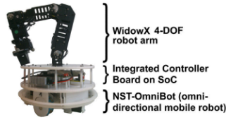
Fig. 1. The mobile manipulator used in our work. The omnidirectional mobile platform is driven by a microcontroller LPC2103 (single core and no floating point unit) running at 64 MHz, whereas the 4-DOF robot arm is driven by a low cost SoC (Zynq-XC702 from Xilinx) running at 100 MHz.
