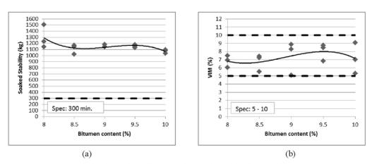
Figure 2. Relationships of stability (a) and VIM (b) with variation of bitumen content.
