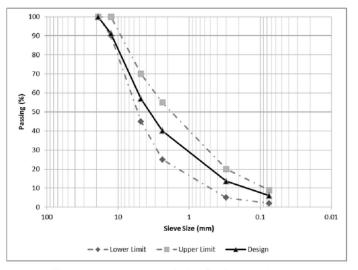
Figure 1. Aggregate gradation for design mixtures.
