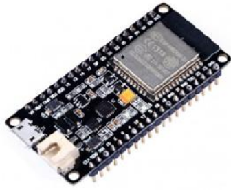
Fig. 2. WEMOS LOLIN32 Lite Bluetooth Low Energy Beacon
