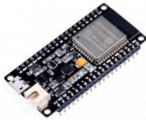
Fig. 2. WEMOS LOLIN32 Lite Bluetooth Low Energy Beacon
