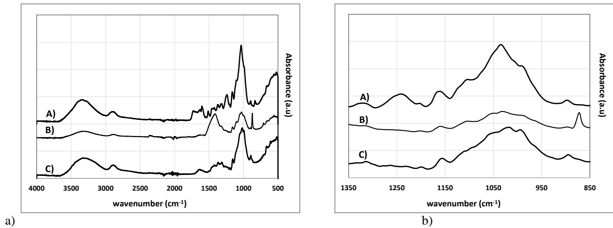
FIGURE 1. FTIR Spectra of a) in 500-4000 \text{cm}^{-1} region and b) in 850-1350 \text{cm}^{-1} region with A) untreated bagasse fibers, B) treated bagasse fibers using \text{Ca}(\text{OH})_2 solution and C) treated bagasse fibers using \text{NaOH} solution
