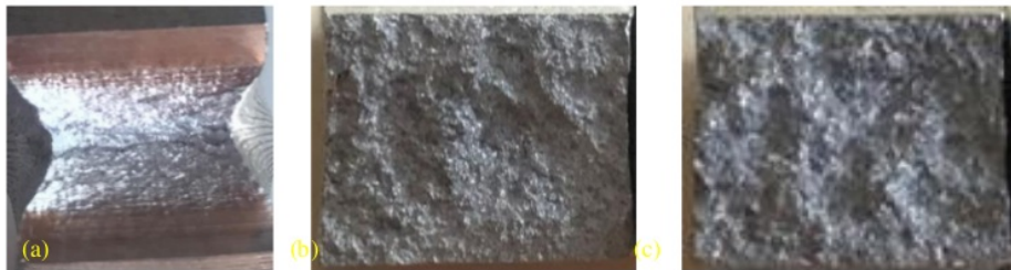
Figure 8. Fracture surface of specimens after impact test a) 0.12 %wt Fe, b) 0.16 %wt Fe, c) 0.20 %wt Fe
