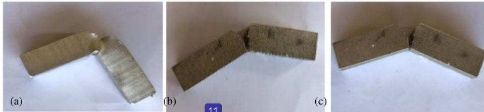
Figure 7. Side view of specimens after impact test a) 0.12 %wt Fe, b) 0.16 %wt Fe, c) 0.20 %wt Fe
