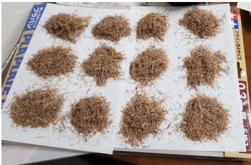
Fig. 3 A mixture of bagasse and rice husk was placed on top of PLA sheet to make a sandwich
