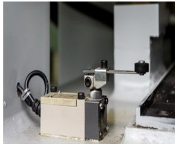
Figure 2. Limit switch as a contact is used to detect objects as machine control
