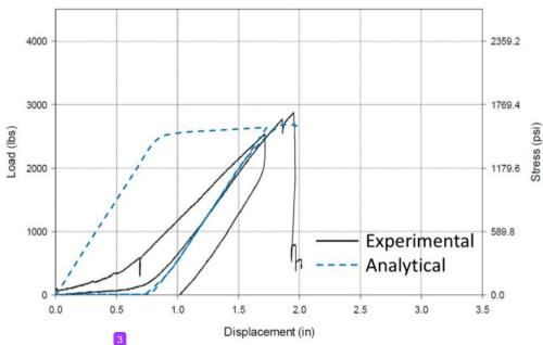
Figure 5. Load-displacement curves of specimen 1SR-S-0.
