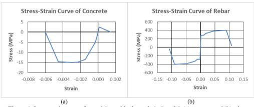
Figure 4. Stress-strain curve of materials used in the analytical model: (a) concrete and (b) rebar.
