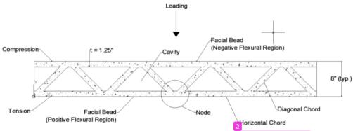
Figure 1. Longitudinal view of 3DCP RC beams tested by Al-Chaar et al. [12].
