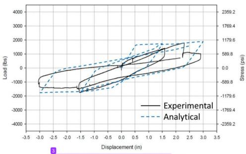
Figure 7. Load-displacement curves of specimen 5DR-B-0.
