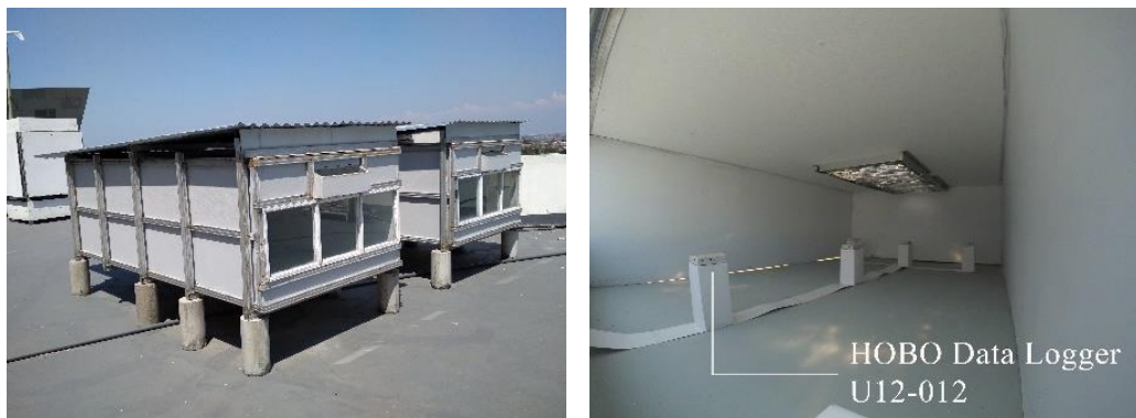
Figure 3. Physical scaled model 1:5 to represent office space which are lit by side window and Horizontal Light Pipe with an egg-crate reflector.
