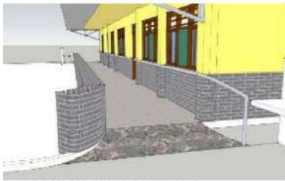
Figure 93 Proposed ramp and railings.
