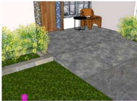
Figure 78 Perspective of front terrace with 1:12-ramp and anti-slip flooring.
