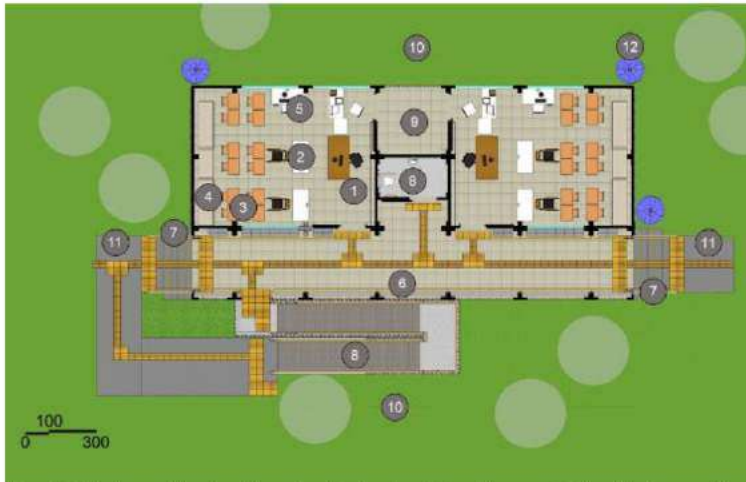
Figure 97 Ideal-accessible school floor plan (Explanation: 1. Teaching area, 2. Wheelchair-accessible seat, 3. Visually impaired seat, 4. Storage lockers, 5. Speaking computer, 6. Corridor, 7. Stairs, 8. Ramp, 9. Storeroom, 10. Greenery).
