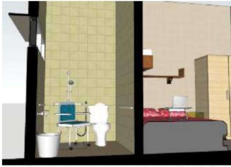
Figure 88 Perspective of bedroom, equipped with anti-slip flooring, bathing chair, sitting toilet, railing, and adjustable shower cap.
