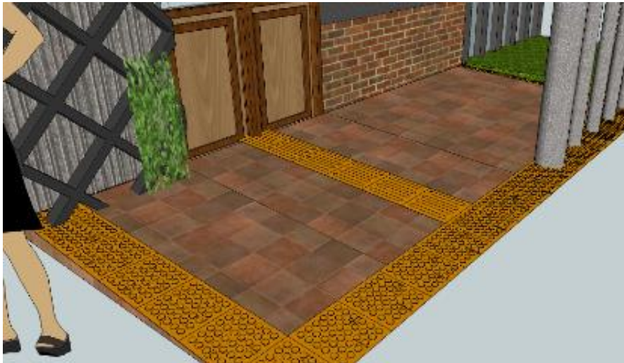
Figure 46 Detail of guiding path in the front terrace.
