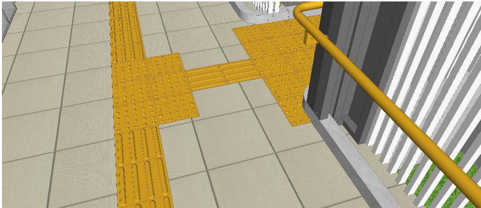
Figure 116 Detail of guiding path in the ideal school ramps.
