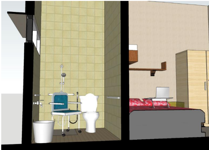
Figure 88 Perspective of bedroom, equipped with anti-slip flooring, bathing chair, sitting toilet, railing. and adjustable shower cap.
