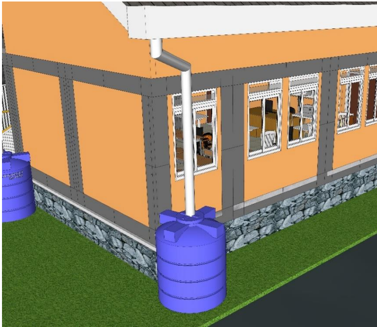
Figure 130 Detail of gutter and water tanks on the ideal school.
