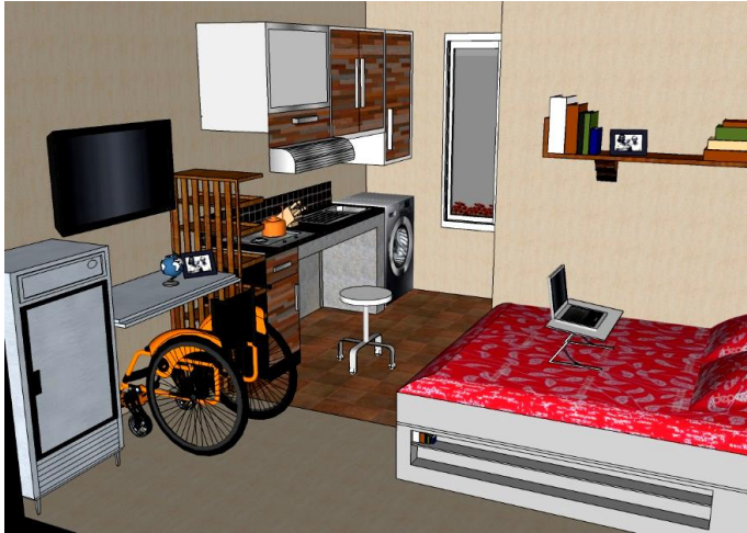
Figure 86 Perspective of working area and pantry that are accessible for wheelchair.
