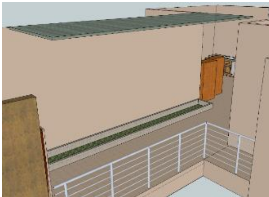
Figure 59 Detail of additional safety railing and canopy.
