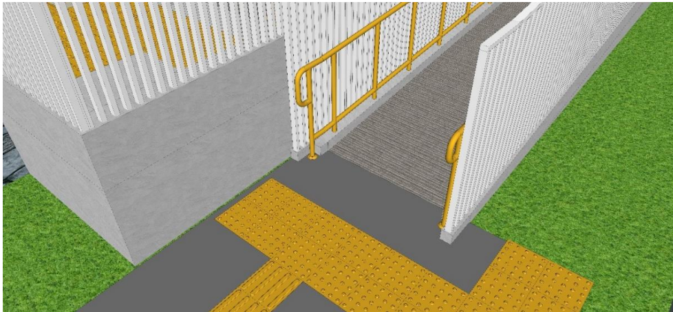
Figure 112 Detail of guiding path in the ideal school ramps.
