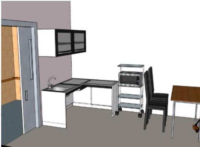
Figure 81 Perspective of kitchen area with wheelchair accessible tops, and anti-slip flooring.
