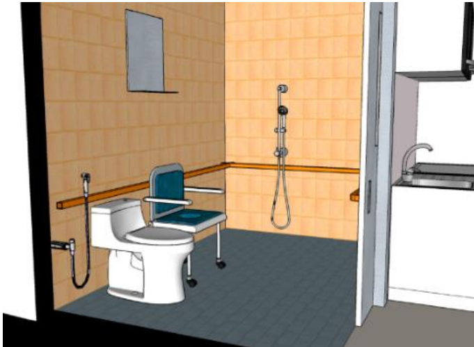
Figure 82 Perspective of bathroom with railing, anti-slip flooring, as well as bathing chair.
