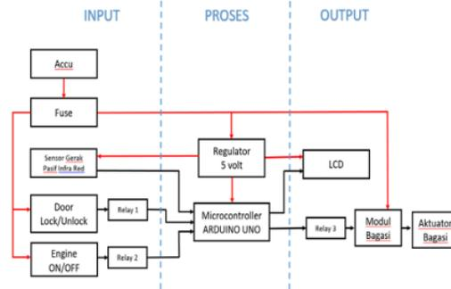
Gbr. 9 Skema wiring diagram
