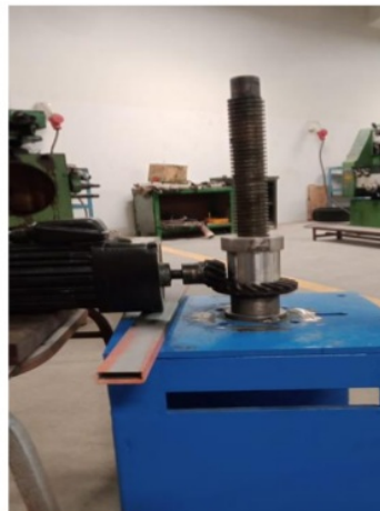
Figure 4. Anvil and pressing mechanism in the design of beverage plastic bottle waste machines
