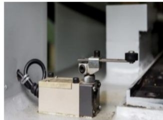
Figure 3. Limit switch as a contact is used to detect objects as machine control
