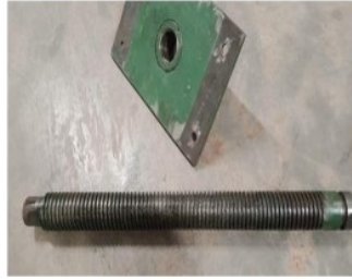
Figure 5. Pressing tool on the design of beverage plastic bottle waste machines
