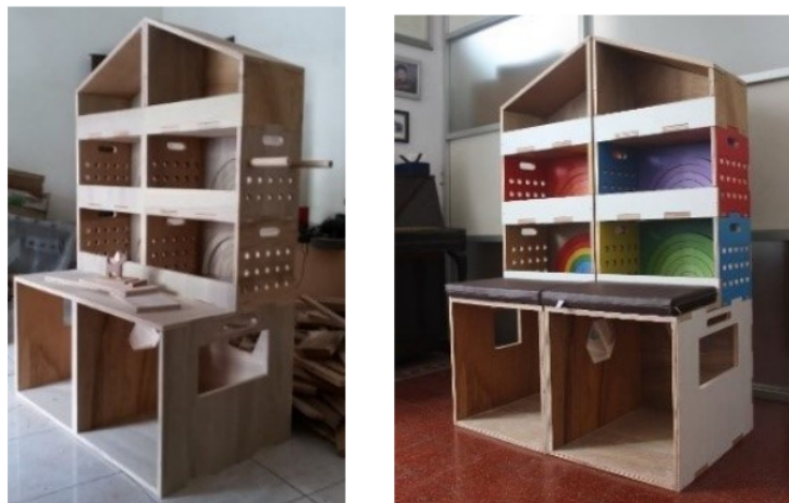
Figure 14. (a) OTTM after CNC Cutting Process; (b) OTTM after Finishing Process
